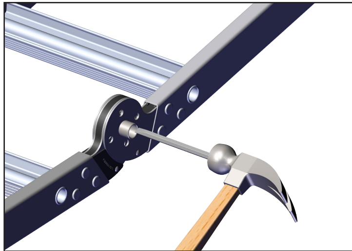
10. If the barrel of the hinge lock remains in the hinge plates, hit the corner of the barrel with a hammer and chisel to remove. Take care not to damage the hinge plate.
